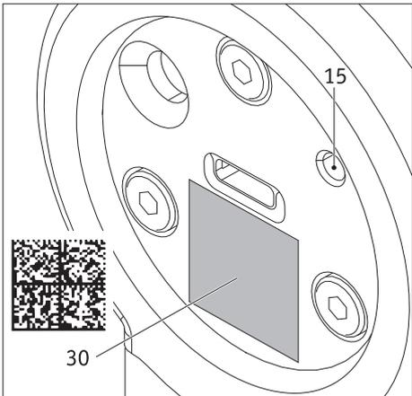
Your SM00V 010 is ready for use again if pairing was carried out successfully. Remove the QR Code from the drive and operating unit and stick them in the user manual for your safety, so that no unauthorized person can connect another control unit to the SM00V 010.
